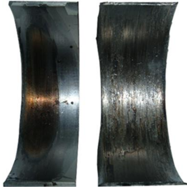
Fig.1 Bearings failed due to oil starvation
