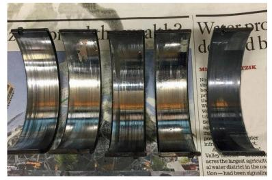
These are five of the lower, uncoated XP bearings as they were pulled directly from the engine after running the test using conventional oil. As you can see, there is considerable wear.
