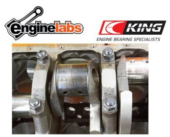
This is what happens when a connecting rod bearing runs for a short time at max load with insufficient lubrication. Connecting rod bearings often fail first because they are heavily loaded and are last in line for lubrication.
