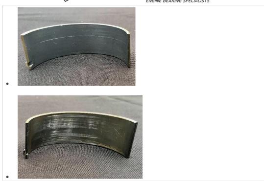
This photo shows the uncoated XP rod bearing on the right after running loaded for over three hours using a 5w20 conventional oil. The same test with the same oil was performed on the King pMaxBlack XP bearing on the left. The wear reduction is obvious.
