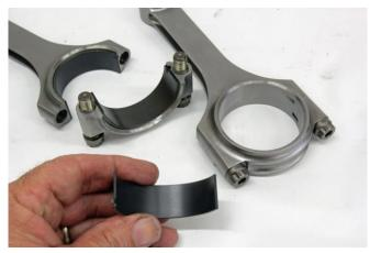
The King pMaxBlack performance bearing isn't a coating but rather a new bearing top overlay that increases hardness by 24-percent yet with 17-percent greater fatigue resistance. Adding the pMax Kote coating makes these bearings even more wear-resistant.
