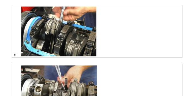
This bearing and oil test demanded the engine be subjected to multiple teardowns to replace all the bearings but the results were well worth the effort. Shavers' small-block has been torn down so many times it should have zippers. To save time, Chrisco changed the main bearings without pulling the crank. He loosened all the main caps and carefully removed the old bearings and installed the new ones by pushing the bearing while turning the crank.
